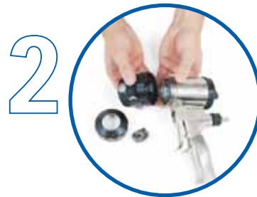
Remove the fluid section from the gun
