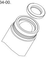
**16.** Gently set P/N P33-11 through P/N 18289-00 Tie Rods and push down square and firm until it sets down over cylinder O-Ring.
