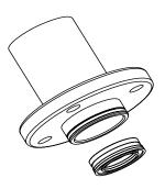
**4.** Lubricate and install O-Ring, P/N <u>13867-43</u> on bottom groove.
