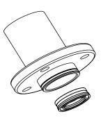
c. Remove Snap Ring, P/N 1005-02, Nylon Washer, P/N 21896-01, & Felt Wipers, P/N 21897-01.
