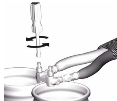
FIG. 21: Open Manual Valves
