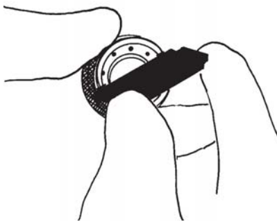
FIG. 27: Unthread Cap from PCD Body
