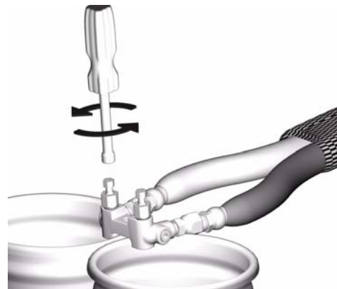
FIG. 13: Open Manual Valves
